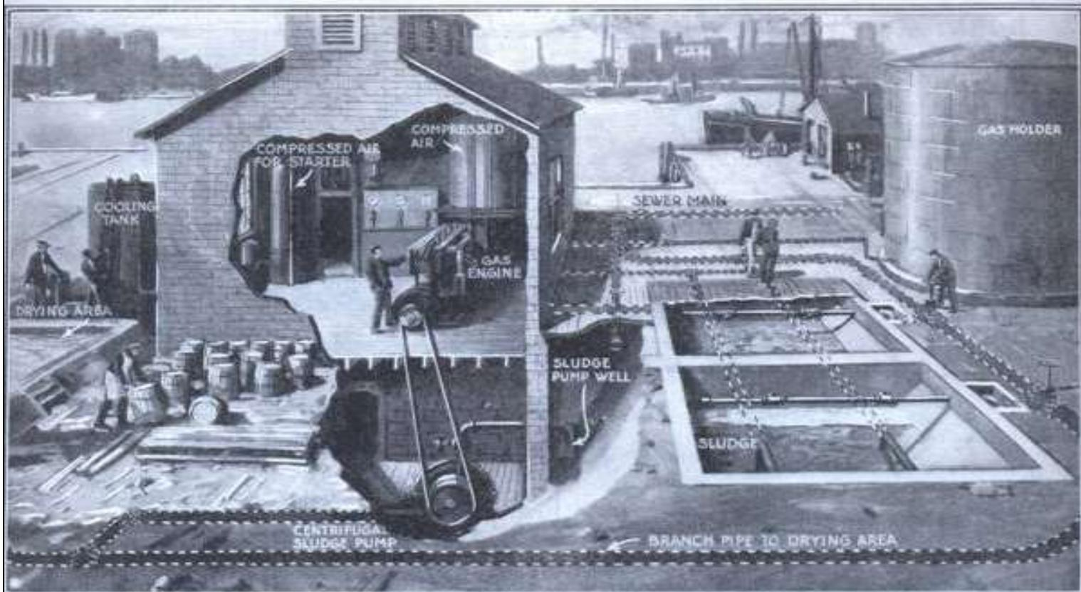
How the sewage disposal plant at Birmingham, England, supplies its own power is described in the illustration. Gas from the sewage drives an engine of 20 brake horsepower, which operates a centrifugal sludge pump
